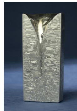
Pure aluminum with columnar grains
