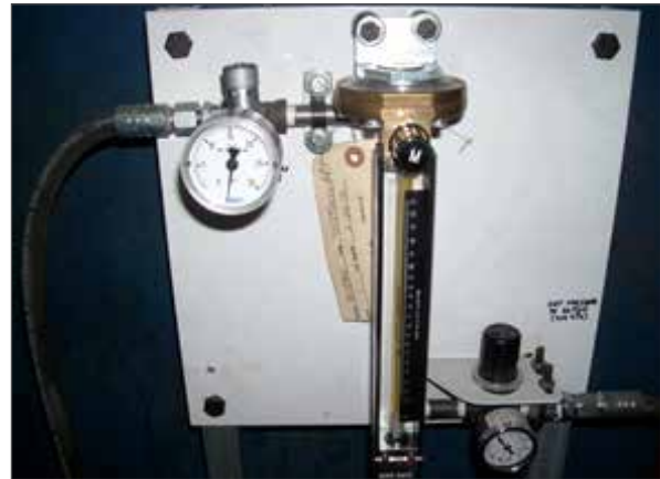
Figure 5. Ancillary components for purging systems
