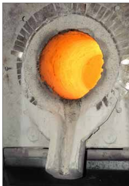
Figure 2. KELLUNDITE lining after furnace tapping
