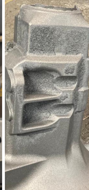
Casting from uncoated mould
