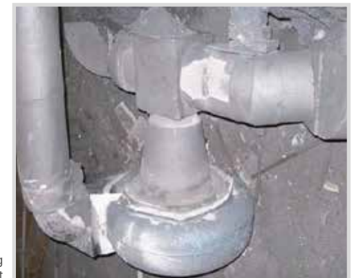
Cast gating system including HOLLOTEX CFU 7 unit
