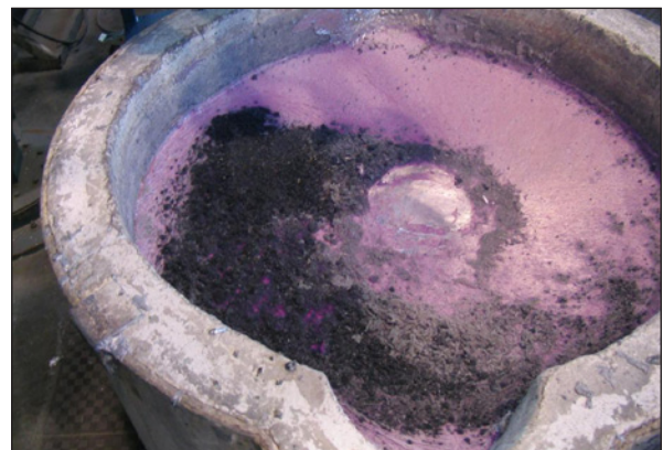
Figure 4. After the MTS 1500 treatment is complete a dry dross remains, significantly reducing the aluminium loss during treatment
