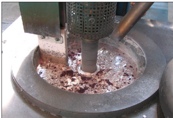
Figure 3. Flotation and degassing proceeds
