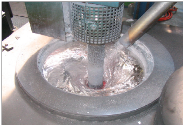
Figure 2. The Vortex has been formed and the flux is dispensed deep into the melt
