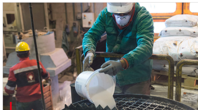
VESBOND 4000 binder addition into the mixer
