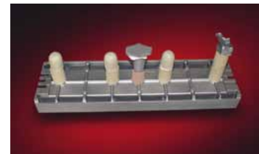
Figure 2 shows a 31.5 kg sand casting with a yield of 75% poured through a KALPUR unit
