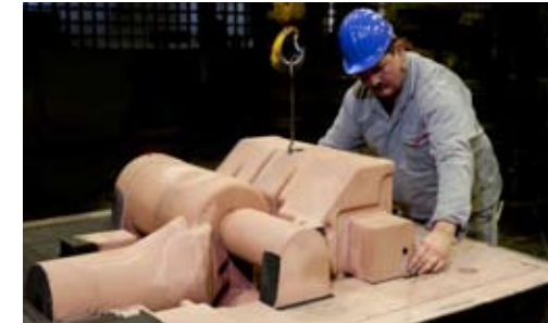
Mould and core package made with REFANOL binder
