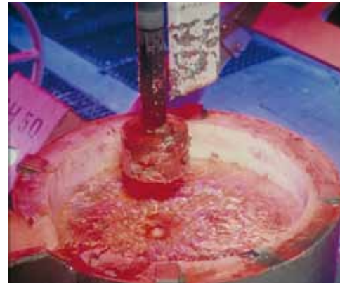
High insulating properties of INSURAL ATL facilitate full metal treatment in the transfer ladle
