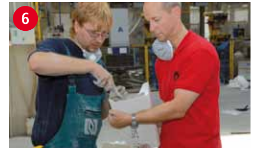
INSURAL 800 mastic is applied to the spout
