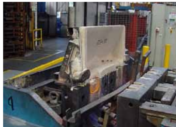
Pouring basin to fill the mould
