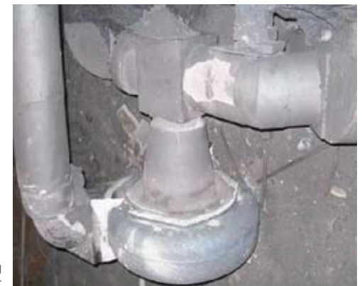
Cast gating system including HOLLOTEX CFU unit
