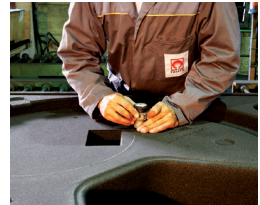
Strength check on cured mould and core
