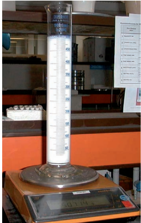
Figure 12: Density measured by weight and volume
