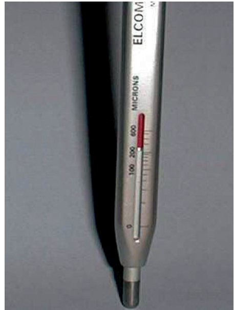
Figure 16: Magnetic system „Pull off Gauge 157“ Elcometer Instruments Ltd. Manchester
