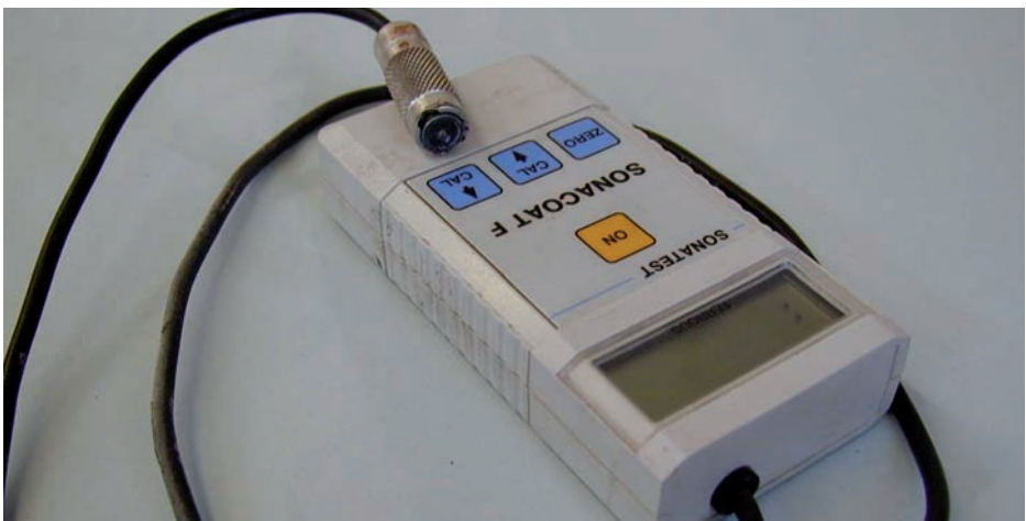
Figure 17: Ultrasonic system Sonacoat F
