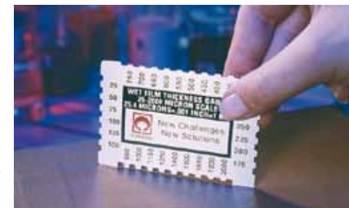
Wet layer coating thickness measurement
