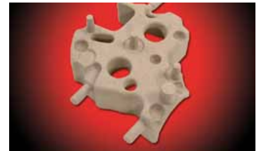
Complex core made with POLITEC binder
