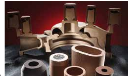
Casting with Foseco sleeves
