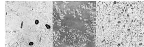
Different structures of a sodium modified AlSi alloy
